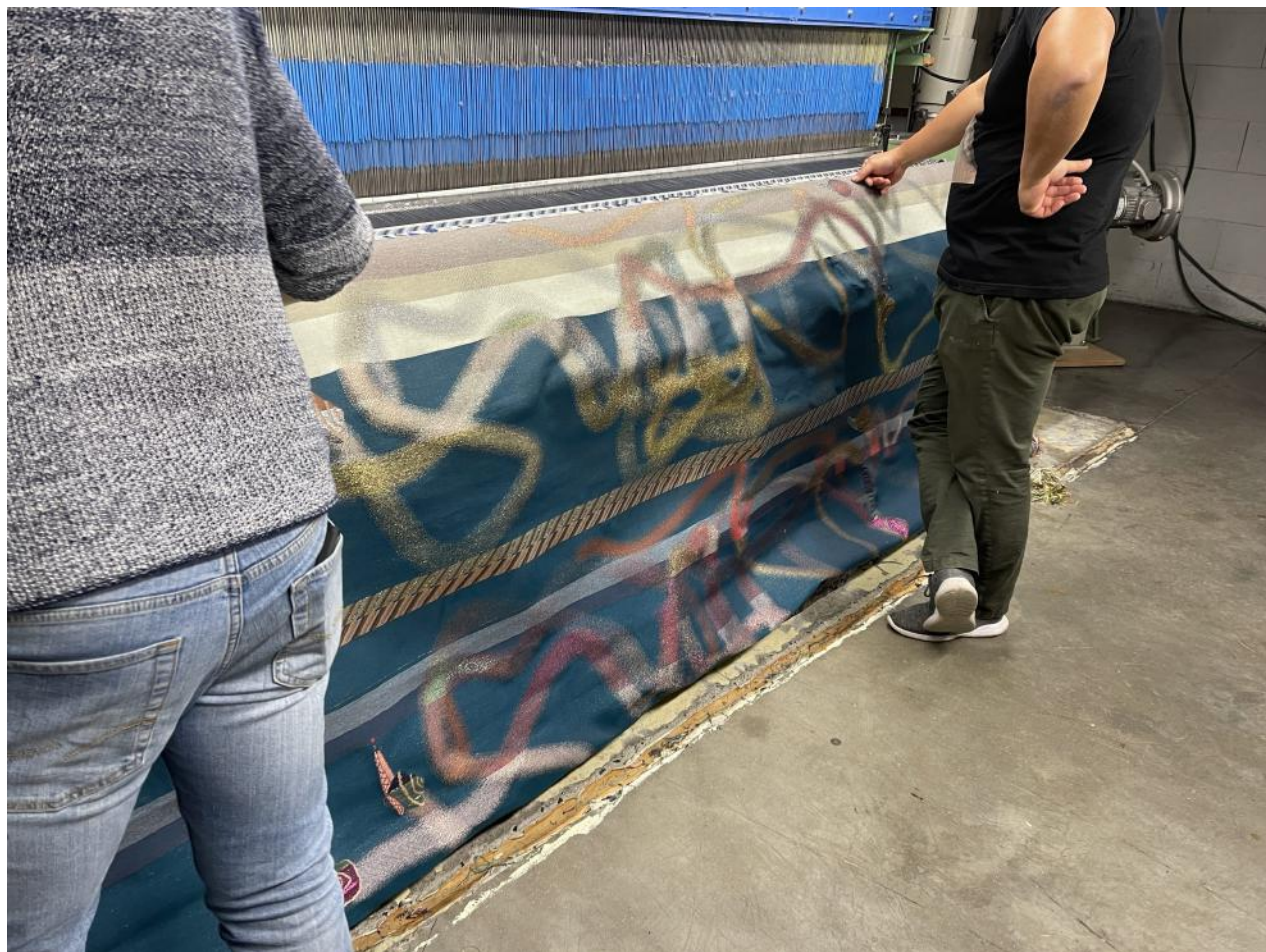
A Jacquard loom at work on a Pae White tapestry. Photo courtesy of the artist.
